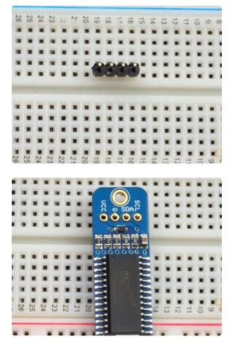
Break off a piece of male header, 4 pins long. Plug the long ends into a solderless breadboard.
