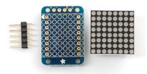
When you buy a pack from Adafruit, it comes with the fully tested and assembled backpack as well as a 8x8 matrix in one of the colors we provide (say, red, yellow or green). You'll need to solder the matrix onto the backpack but its an easy task.
