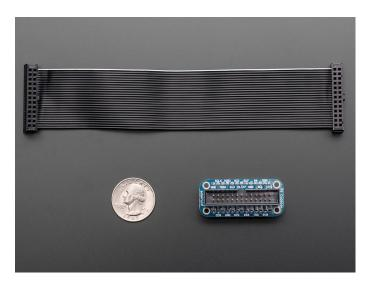
This Cobbler is in a compact shape, which is the least bulky way to wire up.
