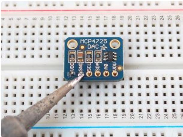
Solder each pin using a soldering iron and solder, to make solid connection on each pin.
