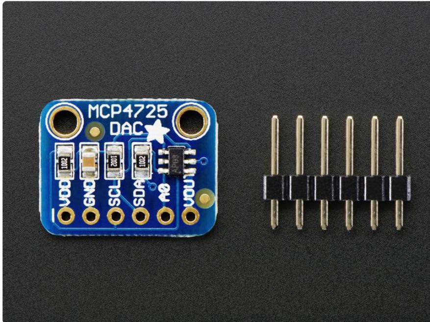
Your microcontroller probably has an ADC (analog -> digital converter) but does it have a DAC (digital -> analog converter)??? Now it can! This breakout board features the easy-to-use MCP4725 12-bit DAC. Control it via I2C and send it the value you want it to output, and the VOUT pin will have it. Great for audio / analog projects, such as when you can't use PWM but need a sine wave or adjustable bias point.
