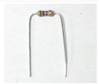
Next, we will solder all of the many resistors. The 10K resistor **R6** is first.
