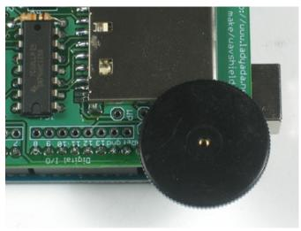
Next you can install the thumbwheel. Use a #0 screwdriver. Align the thumbwheel so it 'grabs' the potentiometer, then gently screw it in place.
