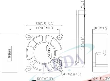
LEAD WIRES: UL 1571, AWG28, L = 140 +/- 10 mm Red = positive; Black = negative.
