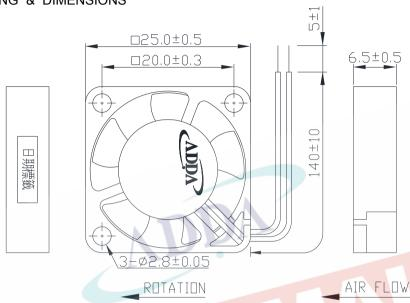
LEAD WIRES : UL 1571, AWG28, L =  $140 \pm 10$  mm Red = positive ; Black = negative.
