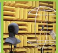
Semi-anechoic chamber According ISO 3744 According ISO 3745 According ISO 7779
