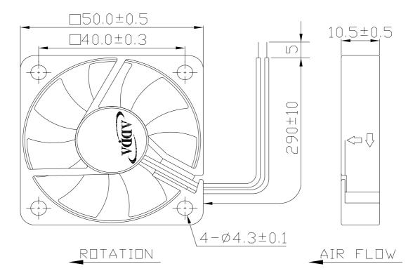
LEAD WIRES: UL 1007, AWG26, L = 290 +/- 10 mm Red = positive; Black = negative.
