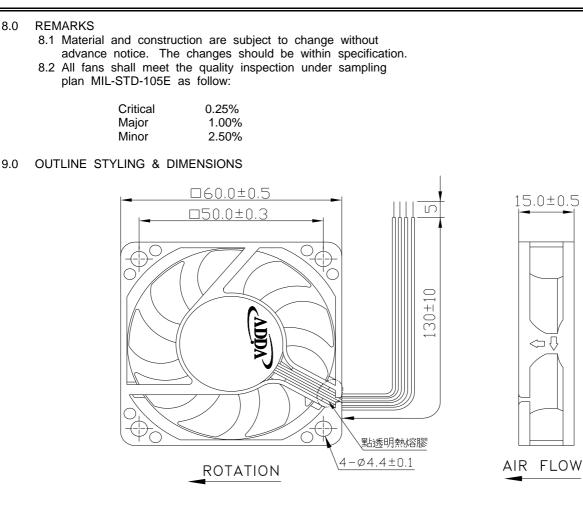
LEAD WIRES : UL 1061, AWG26 , L = 130 +/- 10 mm Red = positive; Black = negative. White = FG ; Blue = pwm input
