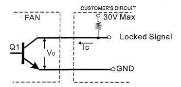
\*Transistor Q1 at "ON" position Collector current....... $I_c$ =10mA Max Saturation Voltage...... $V_{oL}$ =1.0V Max (Between Collector and Emitter at  $I_c$ =10mA) \*Transistor Q1 at "OFF" position Release Voltage...... $V_{OH}$ =30V Max
