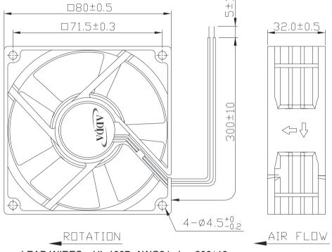
LEAD WIRES: UL 1007, AWG24, L = 300±10 mm Red = positive; Black = negative.
