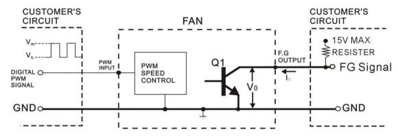
\*TRANSISTOR Q1 AT "ON" POSITION
