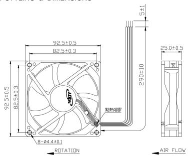
LEAD WIRES : UL 1061, AWG26 , L =  $290\pm10$  mm Red = positive ; Black = negative. White = FG ; Blue = PWM
