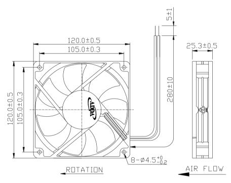
LEAD WIRES : UL 1007, AWG24 , L =  $280\pm10$  mm Red = positive ; Black = negative.
