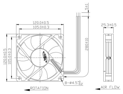
LEAD WIRES: UL 1007, AWG24, L = 280±10 mm Red = positive; Black = negative. White = FG
