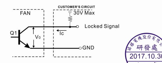
\*Transistor Q1 at "ON" position Collector current.....I<sub>c</sub>=10mA Max Saturation Voltage.....V<sub>oL</sub>=1.0V Max (Between Collector and Emitter at I<sub>c</sub>=10mA) \*Transistor Q1 at "OFF" position Release Voltage.....V<sub>OH</sub>=30V Max
