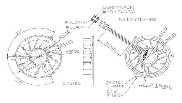
LEAD WIRES: UL 1571, AWG28, L = 80 +/- 10 mm Red = positive; Black = negative. Yellow = FG ; White = pwm input
