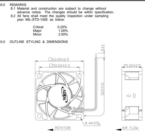
LEAD WIRES : UL 1061, AWG26 , L = 320 +/- 10 mm Red = positive ; Black = negative.
