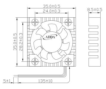
LEAD WIRES: UL 1571, AWG28, L = 135 +/- 10 mm Red = positive; Black = negative.
