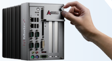
1. Undo the thumbscrew by hand
