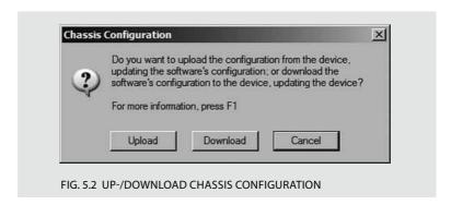
Attention: First of all the user should always initiate an upload before starting any setting-up operation (DeviceNet scanner and bus module).
