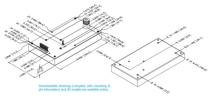
8kV to 30kV High Voltage Cap-Charging Supplies
