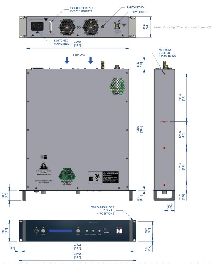
OUTPUT AND ORDERING INFORMATION Model Output Voltage Output Current OL600W-102\* 1 kV 600 mA 5 kV OL600W-502\* 120 mA OL600W-103\* 10 kV 60 mA 20 kV 30 mA OL600W-203\* OL600W-303\* 30 kV 20 mA 40 kV OL600W-403\* 15 mA OL600W-503\* 50 kV 12 mA OL600W-603\* 60 kV 10 mA 80 kV\*\* 7.5 mA OL600W-803\*
