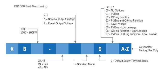
**Example 1:** XB1000-24N-000 = Suitable for BF-rated applications 1000 W, 24 V, output with no options
