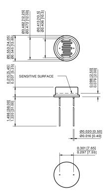
Note: Lead soldering temperature (0.08 inches away from body) 260°C for 5 sec.
