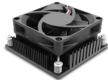
ATS-61700W-C2-R0 74.0 x 74.0 x 24.5mm Thermal Resistance: 0.44°C/W
