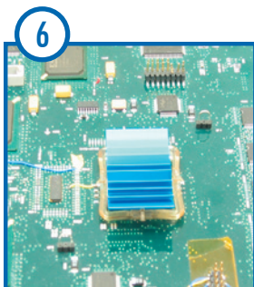
Place the Heat Sink squarely in the Frame Clip over the component. Note the direction of air flow when placing your Heat Sink.
