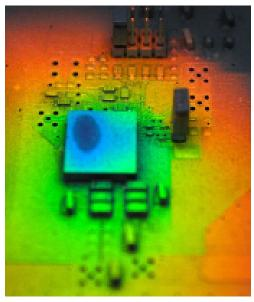
The temperature map of the component is shown after being sprayed with liquid crystals.
