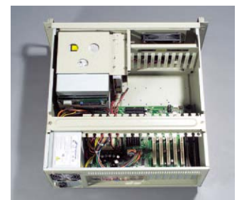
Motherboard can fit in 450 mm (17.7") depth
