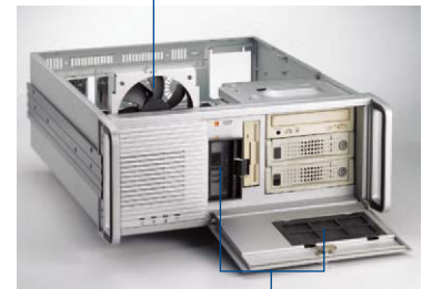
Reusable and easy-to-maintain fan filters
