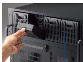
Four hot-swap cooling fans with filter
