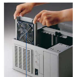
85 CFM easy-to-maintain cooling fan
