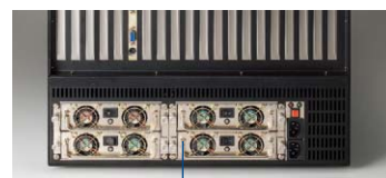
Hot-swap redundant power supply
