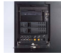
One slim ODD bay, two 3.5" disk drive bays & two removable SATA HDD trays
