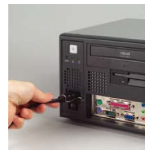
Plug ring-lock securely fastens the power cord
