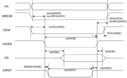
I/O Output (Write) Timing Specification
