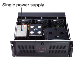
Extra drive bay which can hold up to three 3.5" HDDs
