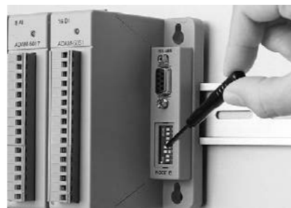
Node ID Setting 8-pin dip switch configuration
