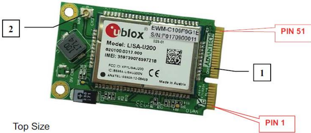
Figure 2-1-3 Appearance of the interfaces on EWM-C109F6 HSPA series module
