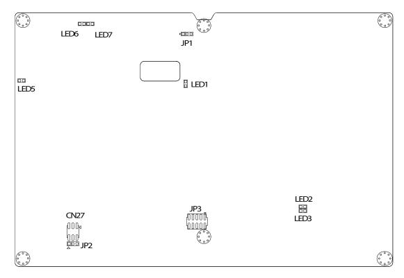
Figure 4.1 Locating Jumpers / LEDs
