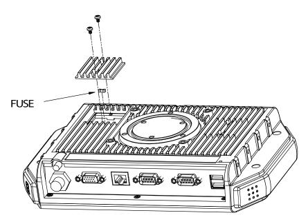
Figure 3.7 Installing the fuse
