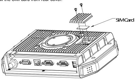
Figure 3.5 Installing the SIM card.
