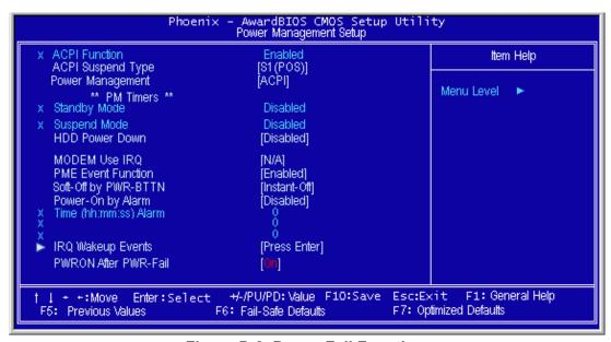
Figure D.2 Power Fail Function
