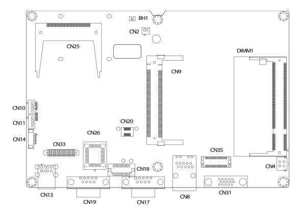
Figure 4.2 Locating Connectors on the front side
