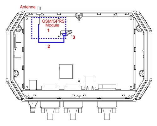
Figure 3.4 GSM / GPRS module
