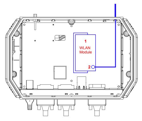
Figure 3.2 MiniPCI Wireless LAN module
