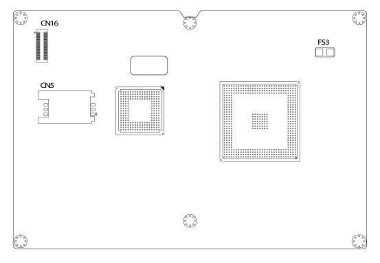
Figure 4.3 Locating Connectors on the back side
