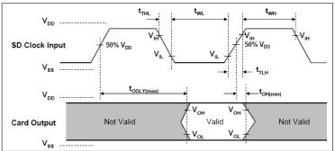
Card Output Timing (High Speed Mode)
