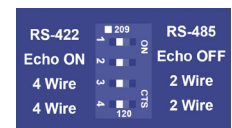
DIP Switch -see Quick Start Guides for configuration details.
