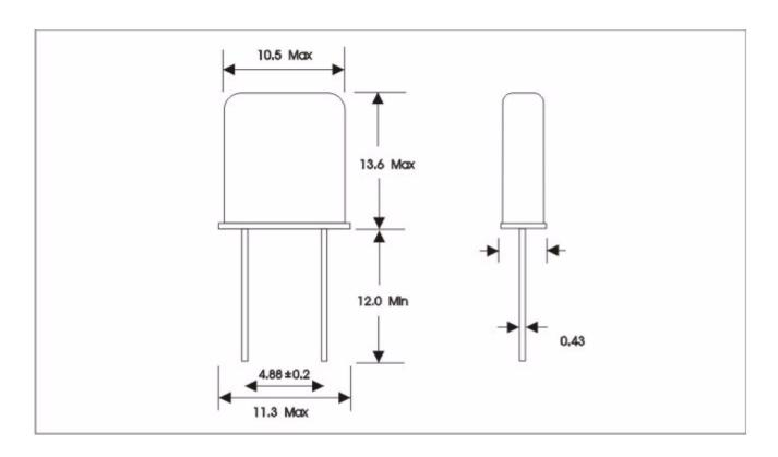
Holder Style Mode Adjustment Tolerance Temperature Stability Operating Temp. Range ESR Marking HC-49/U
