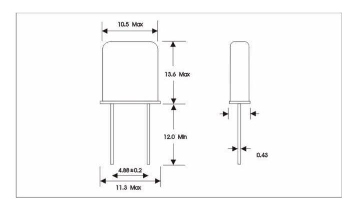
Holder Style Mode Adjustment Tolerance Temperature Stability Operating Temp. Range Load Capacitance ESR Marking HC-49/U
