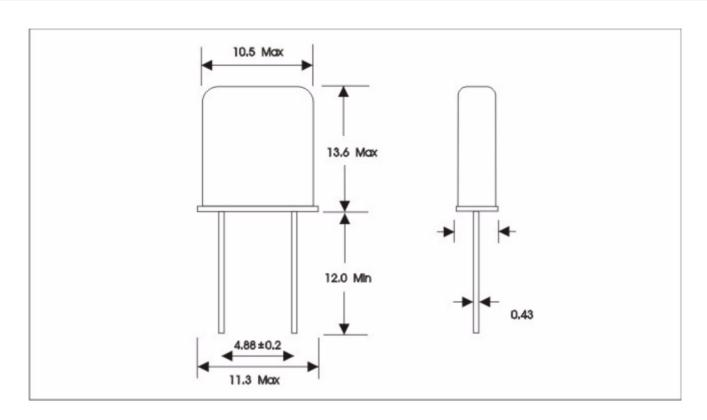
Holder Style Mode Adjustment Tolerance Temperature Stability Operating Temp. Range Load Capacitance ESR Marking HC-49/U Fundamental ± 30PPM at 25°C ± 50 PPM -20°C to +70°C 30 pF 40 Ohm
