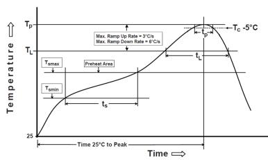
\* Recommended Temperature Profile for Wave Soldering
