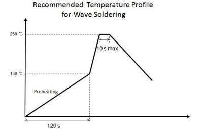
Notice: Wave Soldering is suitable for 1206 and 0603 size.
