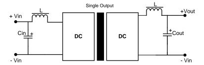
If it is required to decrease the input/output ripple an "LC" filter network can be installed on the input and output of the converter (see above).
