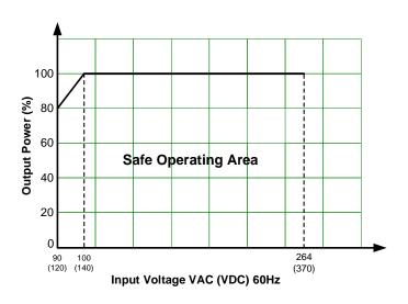
Note: With an AC input voltage between 90-100VAC and a DC input between 120-140VDC the output power must be derated as per the temperature derating curves.
