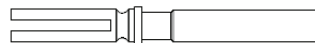
57 Socket, straight, crimp-removable (20–22 AWG) 58 Socket, straight, crimp-removable (24–26 AWG) 59 Socket, straight, crimp-removable (28–30 AWG)
