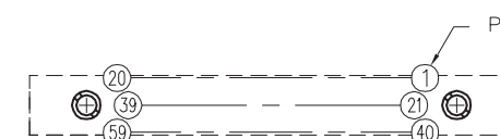
PIN IDENTIFICATION PATTERN VIEWED FROM TERMINATION SIDE
