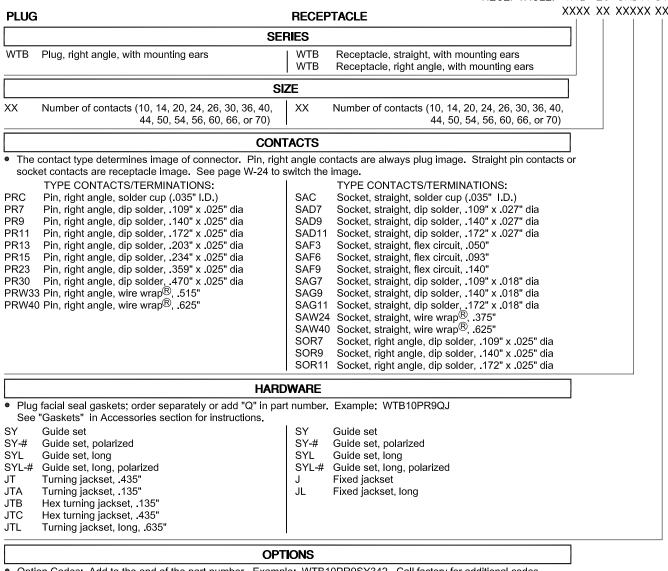
• Option Codes: Add to the end of the part number. Example: WTB10PR9SY342. Call factory for additional codes.
