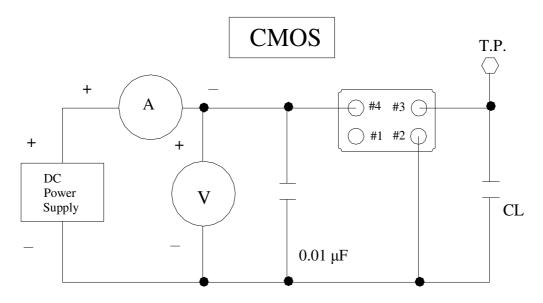
\*\*\*Because SMA series has no by pass capacitor. So,we recommend our customer to use capacitor 0.01  $\mu F$  in join Vcc and GND.
