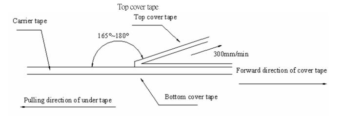
\*\*\* In the case, the cover tape is pulled off under the above conditions, the cover tape adhesion strength should be 10.2g~71.4g Plastic tape: 10.2g~71.4g
