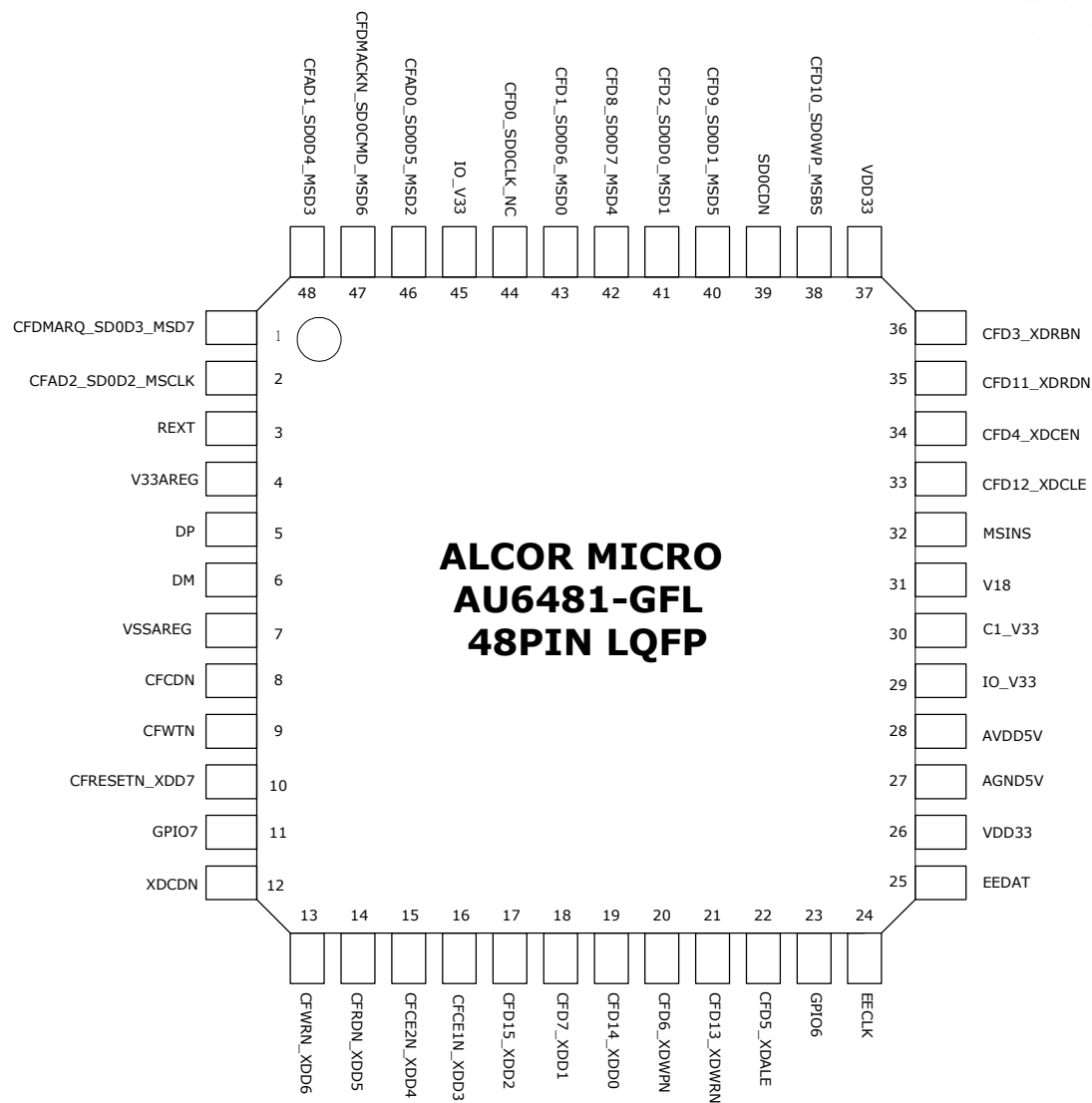
Figure 3.1 AU6481 Pin Assignment Diagram
