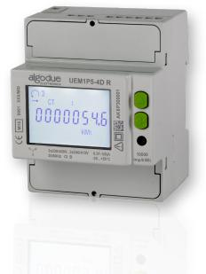
4 DIN modules energy meter for the energy measurement in industrial and civilian application, with the following built-in communication, according to the model: RS485 Modbus RTU/ASCII, M-Bus or Ethernet Modbus TCP. Available with MID certification suitable for billing.
