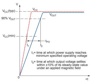
Figure 1: Definition of Power-On Time, t<sub>PO</sub>
