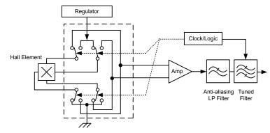
Figure 6: Chopper Stabilization Technique
