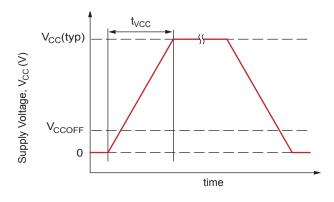
Figure 4: Definition of V<sub>CC</sub> Ramp Time, t<sub>VCC</sub>
