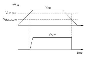
Figure 3: Definition of Undervoltage Lockout
