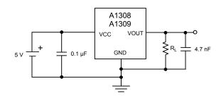
Figure 5: Typical Application Circuit
